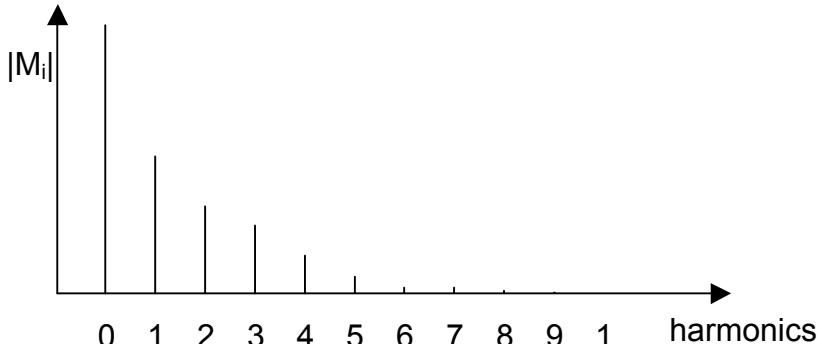
The solution for the zero-order harmonic is obviously Poiseuille's law. Let us now consider the solution for a single harmonic pressure gradient. The general solution would be then a linear addition of Poiseuille's solution for the zero-order term plus the solution for each harmonic. For a single harmonic:
