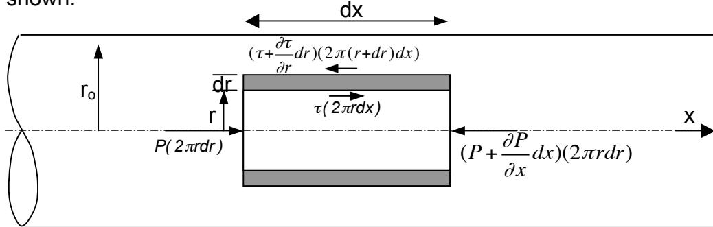
Assuming uniform flow (1<sup>st</sup> assumption), the balance of forces acting on the fluid element in the x-direction yields:
