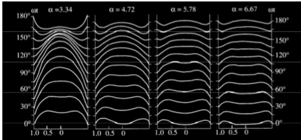
Velocity  $v(r,t)$  can be expressed in terms of amplitude and phase. The velocity profile shows that not all points along the radius move in phase. The phase
