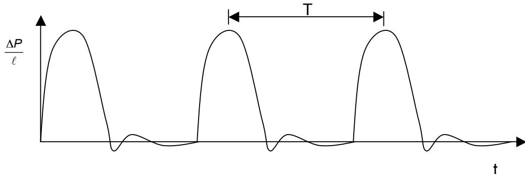
So, if we assume (4<sup>th</sup> assumption) that the pressure gradient  $\frac{\partial P}{\partial x} = \frac{\Delta P}{\ell}$  is a periodic function, with period  $T$ , as shown in the figure above, we can express the pressure gradient in terms of a Fourier series:
